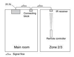
The miniplug cable from the connecting block should be connected to the AV receiver's IR IN jack, as shown below.
